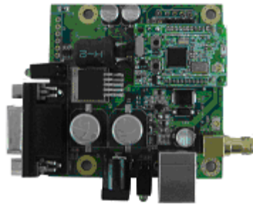
ZigBee-100 Extension Board: for external plug in to existing systems
