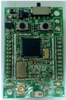
ZigBee-100 Tag: for system integration
